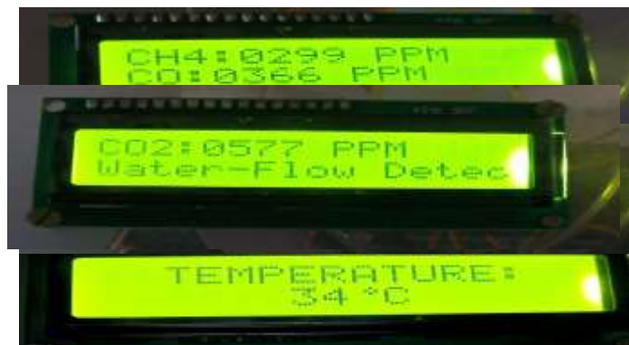
Fig4.4: Abnormal condition data display
