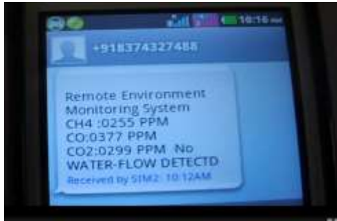
Figure 4.5: Received SMS shows gas levels and water flow is detected info
